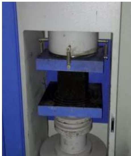
Figure3.Compressive strength test of cube using CTP
